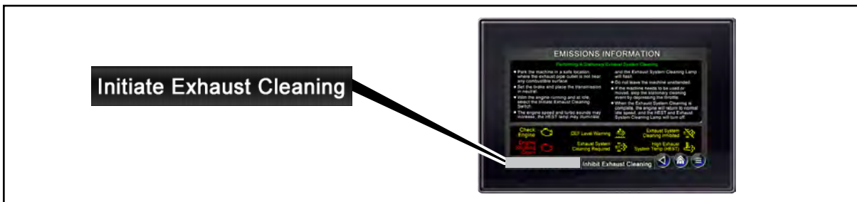
Initiate Exhaust Cleaning Function Button
