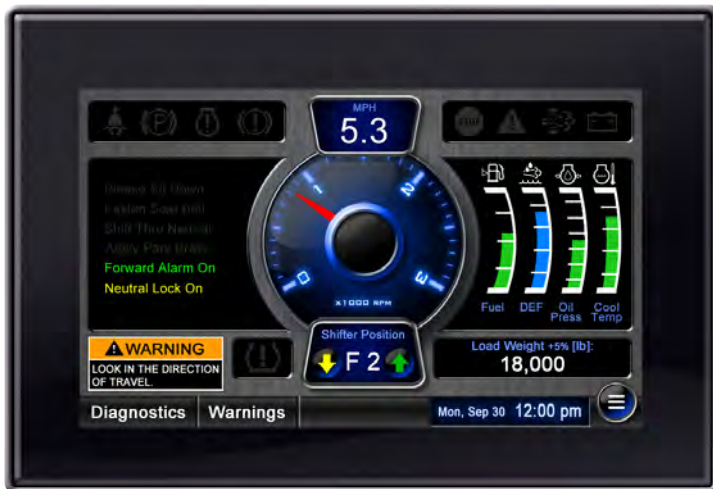
Forward Alarm Operation (Automatic Mode)
