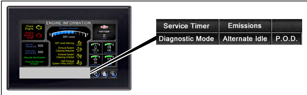
Engine Information Screen Function Buttons
